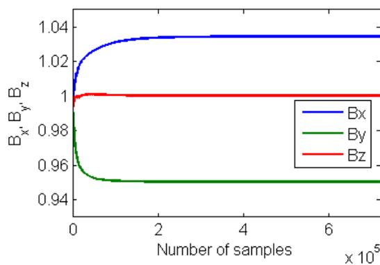
**Figure 5** Learning process of sensitivity calibration constants
