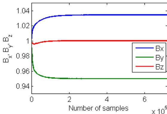
**Figure 13** Learning process of sensitivity calibration constants
