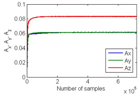
**Figure 14** Learning process of bias calibration constants
