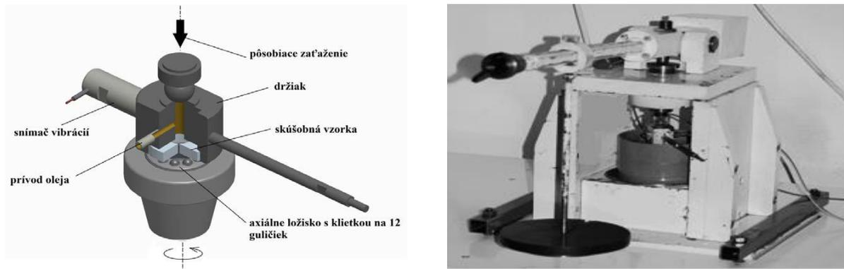
**Fig. 1 a,b** Principle of testing node and AXMAT device
