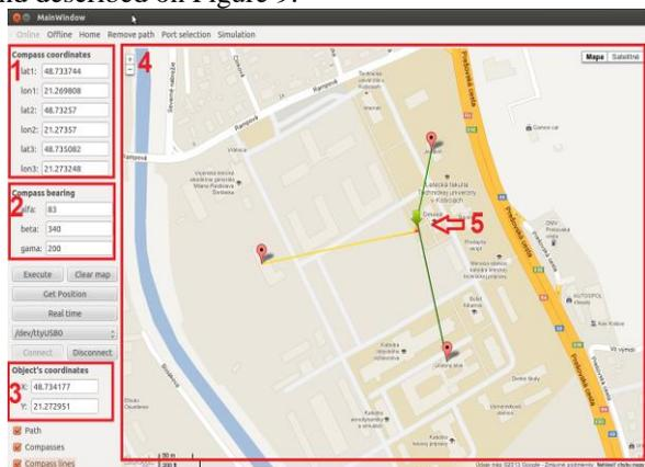
Figure 9 Basic parts of application for object position calculating.
