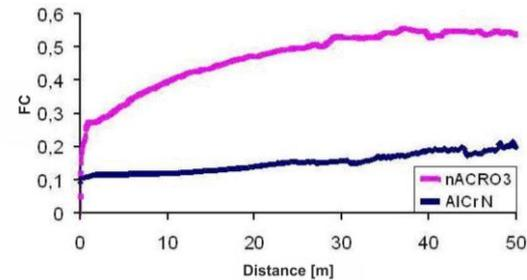
Figure 14 FC for AlCrN and nACRo3 coatings; F=0,5N; ball speed v=10cm/s
