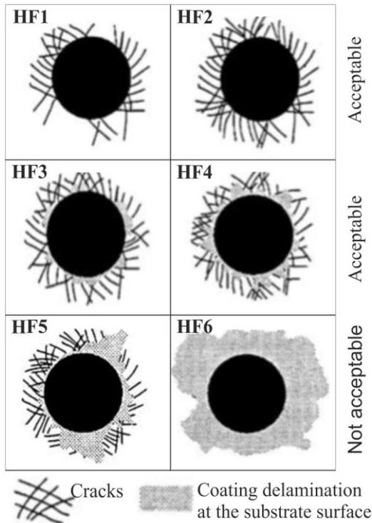
Figure 2 Scale classifying the adhesion by means of Mercedes test [10]
