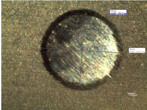
Figure 6 Polished calotte on nACRo3 coating after Calotest, thickness 3.2 μm
