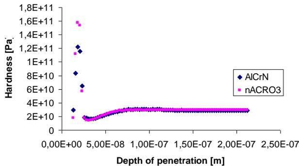
Figure 11 Hardness of CrAlN and nACRo3 coating
