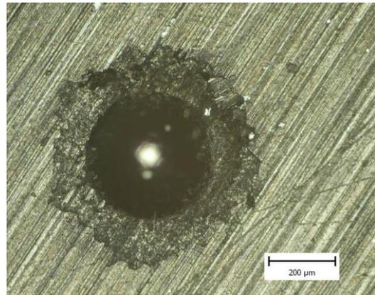
Figure 9 Mercedes test AlCrN coating on steel CPM 10V
