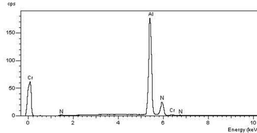
Figure 5 EDX analysis of AlCrN in the point 1.
