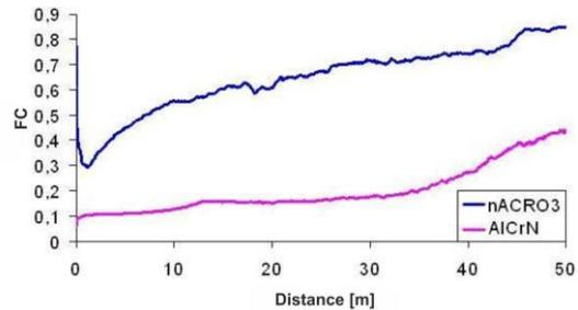
Figure 13 FC for AlCrN and nACRo3 coatings; F=0,5N; ball speed v=5cm/s
