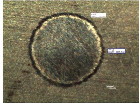
Figure 3 Polished calotte on AlCrN coating after calotest, thickness 1.7 μm.
