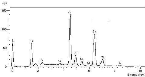
Figure 8 EDX analysis of nACRo3 layer
