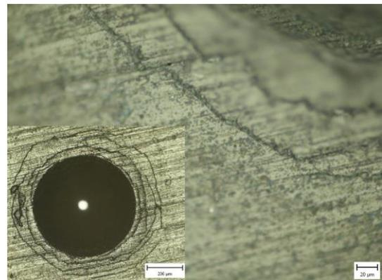
Figure 10 Mercedes test of nACRo3 coating on steel CPM 10V
