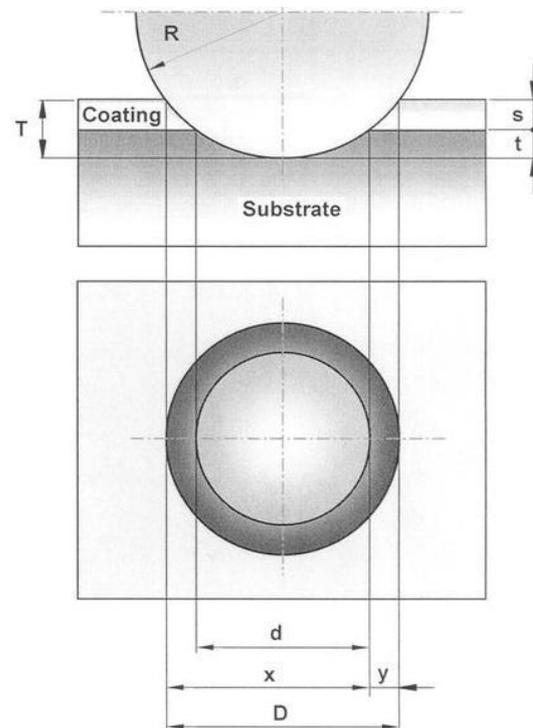
Figure 1 Dimensions of cut-out Calot (based on the standard EN 1071-2).
