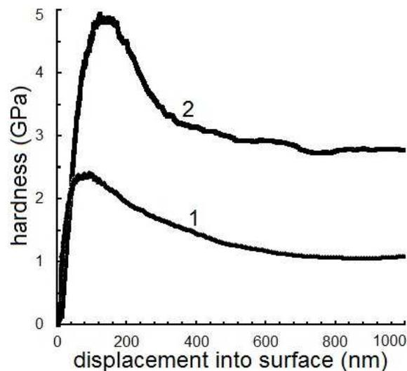
**Figure 7** Hardness of Ti coatings: 1 - 2.4 GPa and 2 - 4.9 GPa
