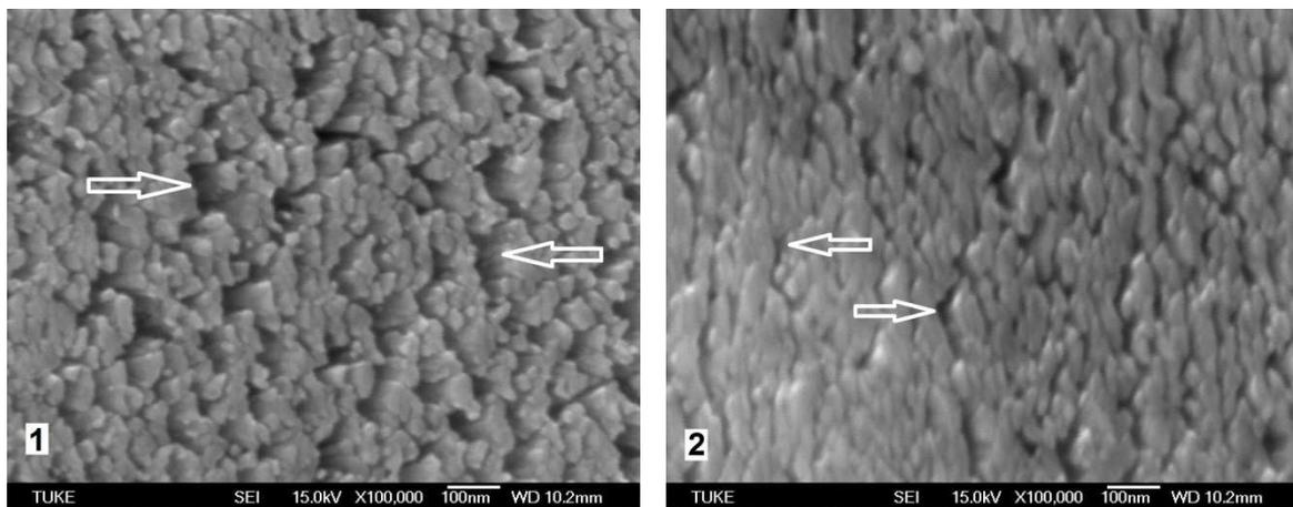
Figure 4 Front view of Ti coating with gaps (see arrows): (1) and (2)
