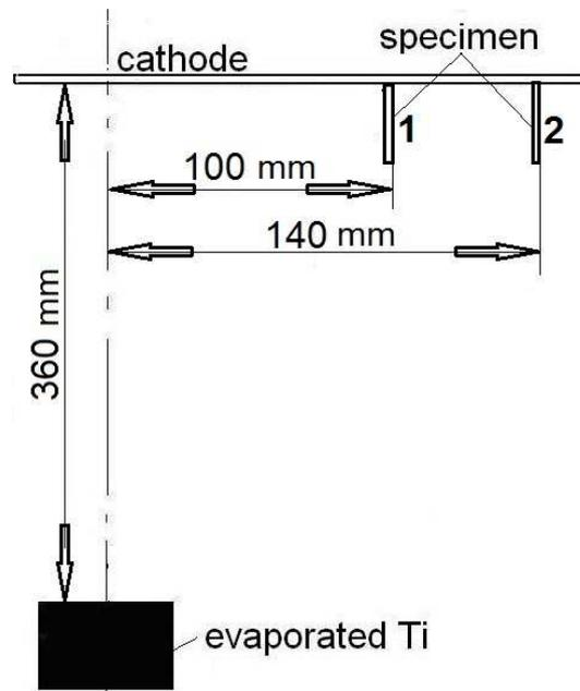
**Figure 2** Locations of samples (1 and 2) inside the vacuum chamber, schematically
