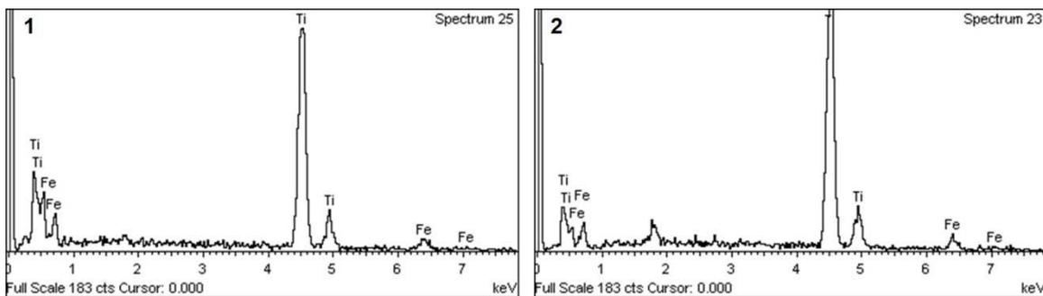
Figure 5 Chemical composition (EDS) of Ti coatings: sample 1 and 2
