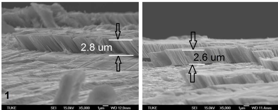
Figure 3 Thickness of Ti coating: (1) 2.8 μm and (2) 2.6 μm
