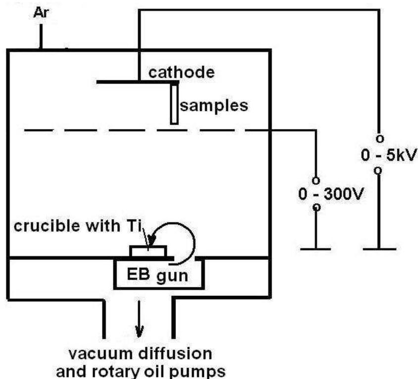
**Figure 1** The apparatus for activated evaporation using electron beam (EB PVD), schematically
