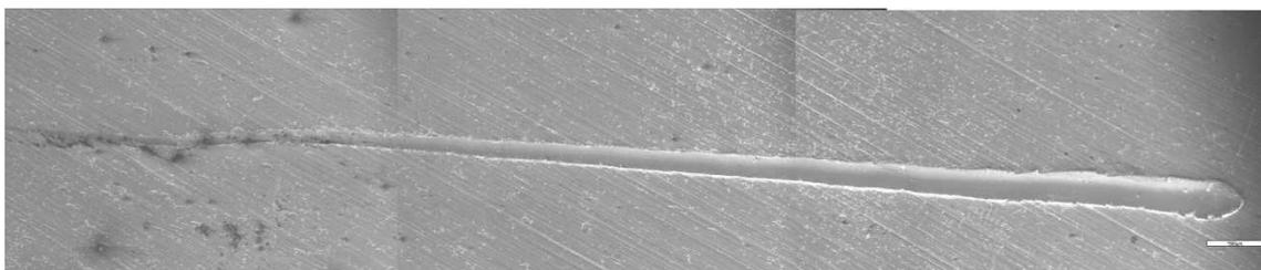
Figure 6 Scratch after Scratch test, coating on the sample 1, adhesion 31 N, total length of scratch 12 mm
