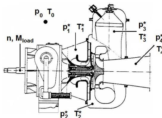
**Figure 1** Longitudinal section of Klöckner-Humboldt-Deutz T216 turbine engine (based on [10])
