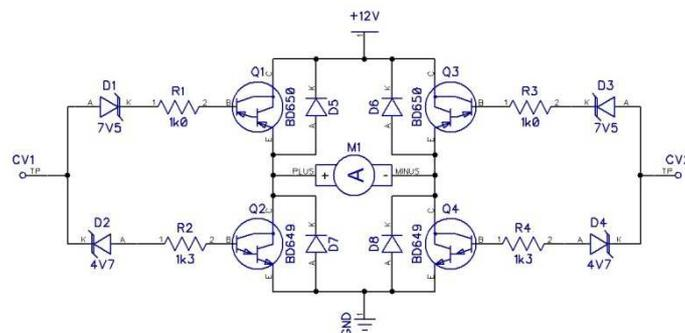
**Figure 3** H-bridge circuit electrical schematic
