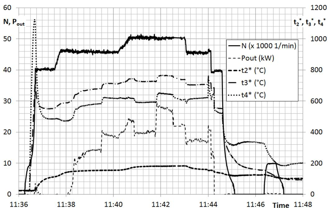
Figure 5 Engine test run temperature and power data
