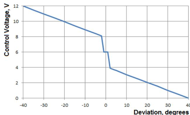
Figure 4 Transfer function of control system
