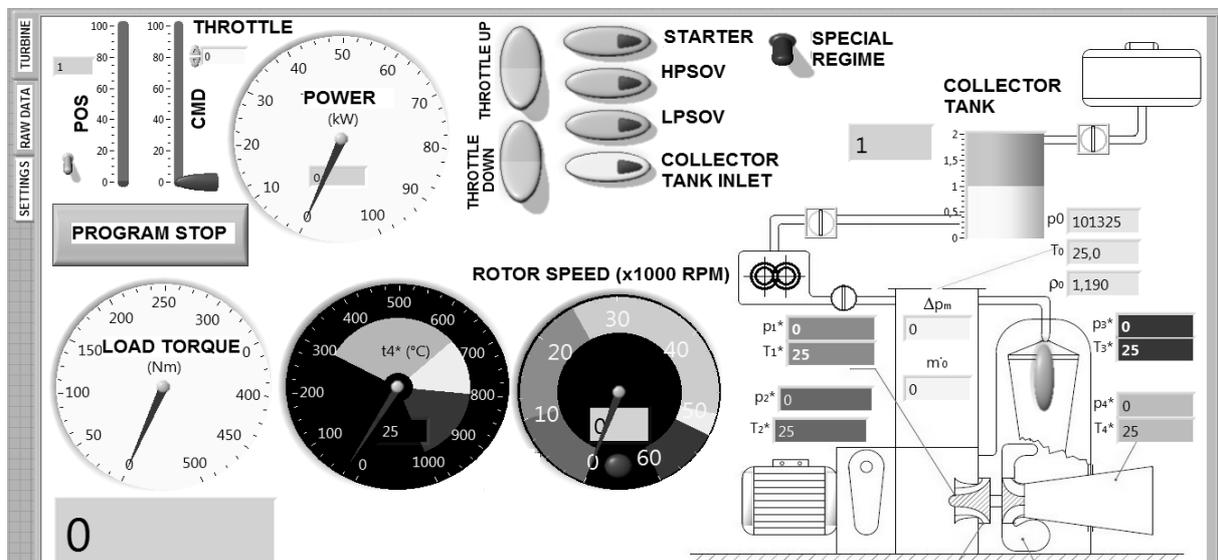
Figure 2 Front Panel of LabVIEW software
